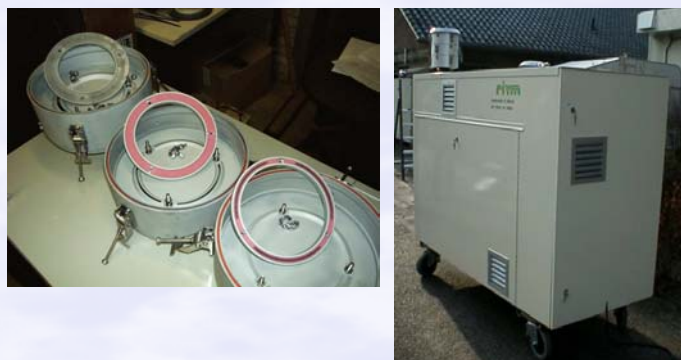
Figure 1: RAIAP PM collection device with the HVCI on top of a box with the pump pull the air through the impactor (right panel) and the inside of the HVCI showing the pink PUF with collected PM (black) of the fine mode stage (left panel).
