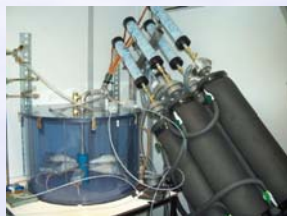
Animal models are being widely used to measure the effects of exposure to air pollution. This figure shows a device used to expose rats to ambient air particles. Afterwards the rats are examined to investigate the possible effects of the exposure.
