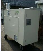
Figure 1: RAIAP PM collection device with the HVCI on top of a box with the pump pull the air through the impactor (right panel) and the inside of the HVCI showing the pink PUF with collected PM (black) of the fine mode stage (left panel).
